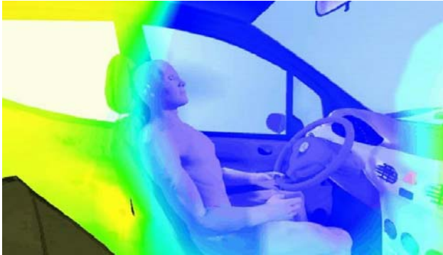
Figure 2: Temperature distribution in a car.
