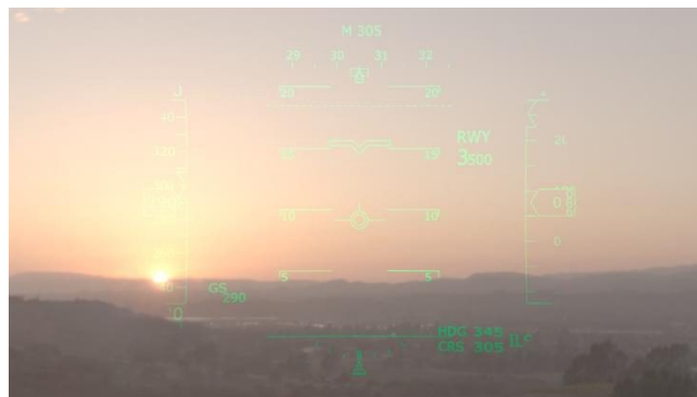
Figure 8. The HUD image simulation result within the real environment in the case of high environment luminance and low HUD light source luminance.
