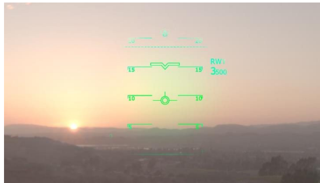
Figure 13. The HUD without an intermediate diffuse screen image simulation result with merged forward and bidirectional stochastic ray tracing methods within the real environment.
