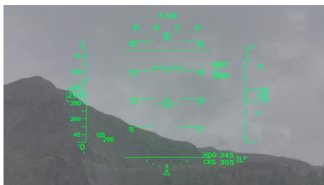
Figure 10. The HUD image simulation result within the real environment in the case of low environment luminance and optimal HUD light source luminance.
