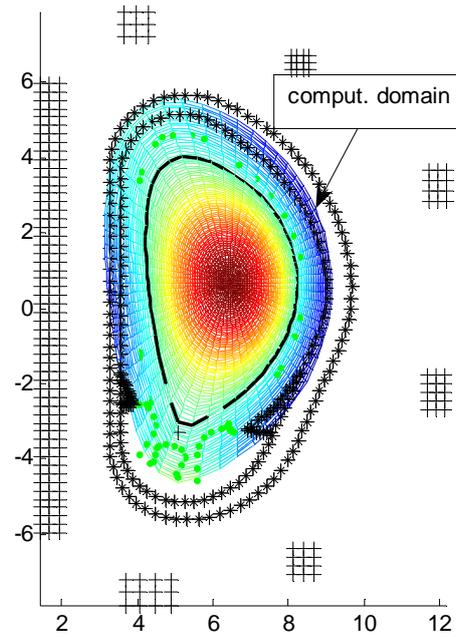
Fig.3a Free boundary plasma equilibrium on magnetic surface adaptive grid.
