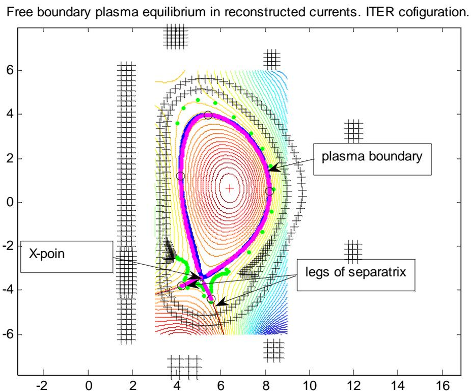
Fig.4 Free boundary plasma equilibrium on rectangular grid in reconstructed currents. ITER configuration.
