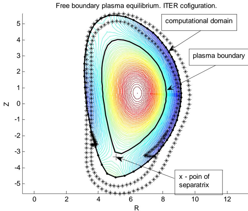
Fig.3b Free boundary plasma equilibrium on magnetic surface adaptive grid.
