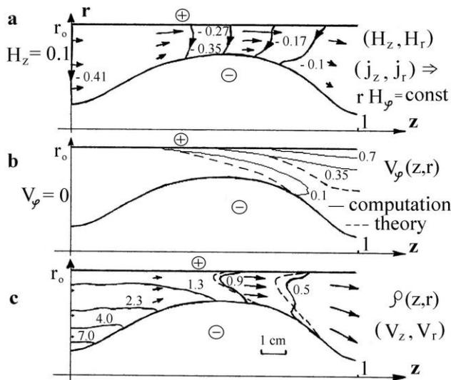
Fig. 1. Plasma flow in the presence of a longitudinal magnetic field: a) electric current  $(j_z, j_r)$  (level lines of the function  $r H_\phi = \text{const}$ ) and vector magnetic field distribution; b) level lines of the ion azimuthal velocity  $V_\phi$ ; c) density distribution  $\rho(z, r)$  and vector velocity field of the ion component  $(V_z, V_r)$ . The broken curve corresponds to the analytical model.
