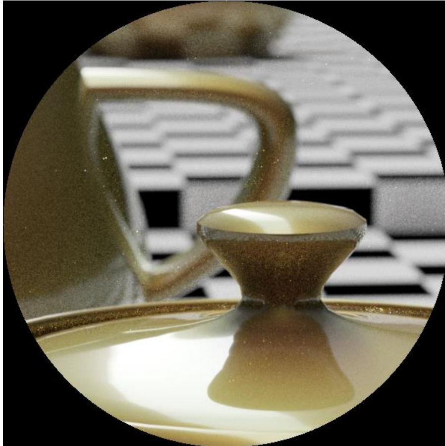
Figure 7. The image viewing in VR system (the left eye) with the shifted LCD and the corrected focal distance of the eyepiece. The eye is accommodated on 565mm
