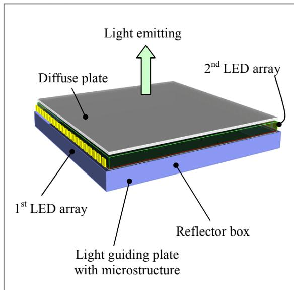
Fig. 1. Scheme of luminaire for indoor illumination
