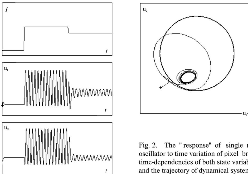
Fig. 2. The "response" of single network oscillator to time variation of pixel brightness: time-dependencies of both state variables (left) and the trajectory of dynamical system (right).
