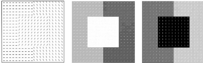
Fig. 4. Segmentation of the image consisting of three fragments of the same brightness but different monodirected texture.
