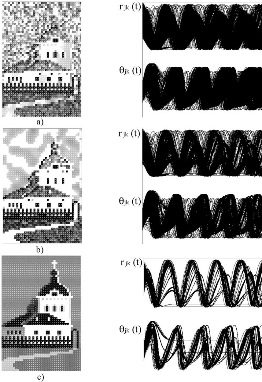
Fig. 3. Three main types of network dynamical behavior that occur in the process of interaction strengthening: a) total desynchronization ( $h=1.25$ ); b) partial synchronization ( $h=0.5$ ); c) almost complete synchronization ( $h=0.01$ ). One of instantaneous network states, mapping current result of image segmentation (left), and time-dependence curves of all oscillator variables (right) are shown.
