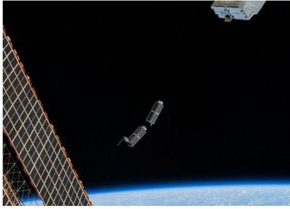
**Figure 2. The photo of the launch of the two Doves PlanetLabs's 3U CubeSats from the ISS [17]**
