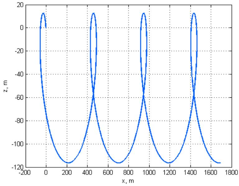
**Figure 4. Free relative motion after the launch**
