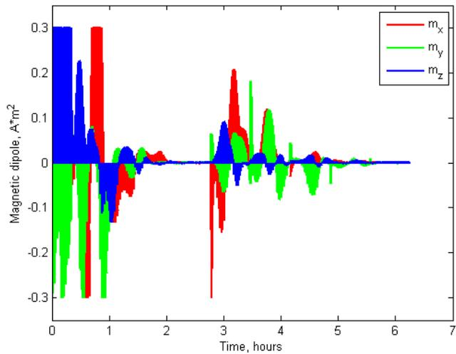
**Figure 8. The magnetorquers control values for the second satellite**
