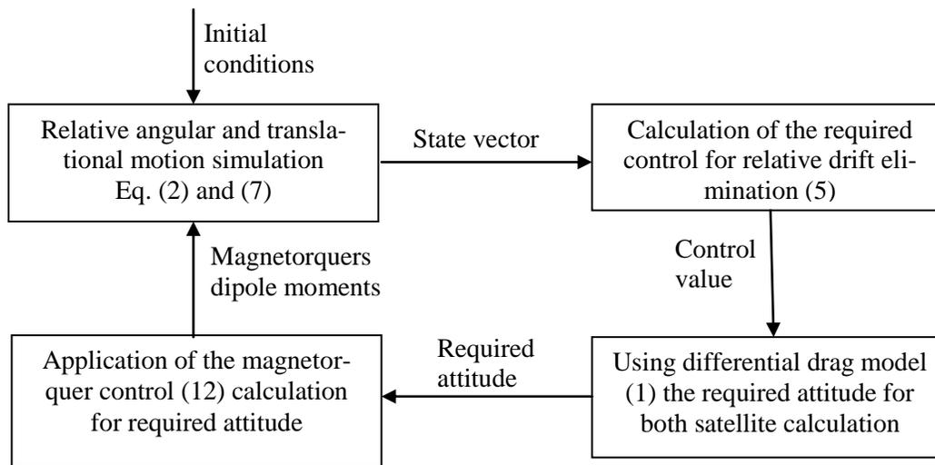
**Figure 3. Scheme of the control loop**
