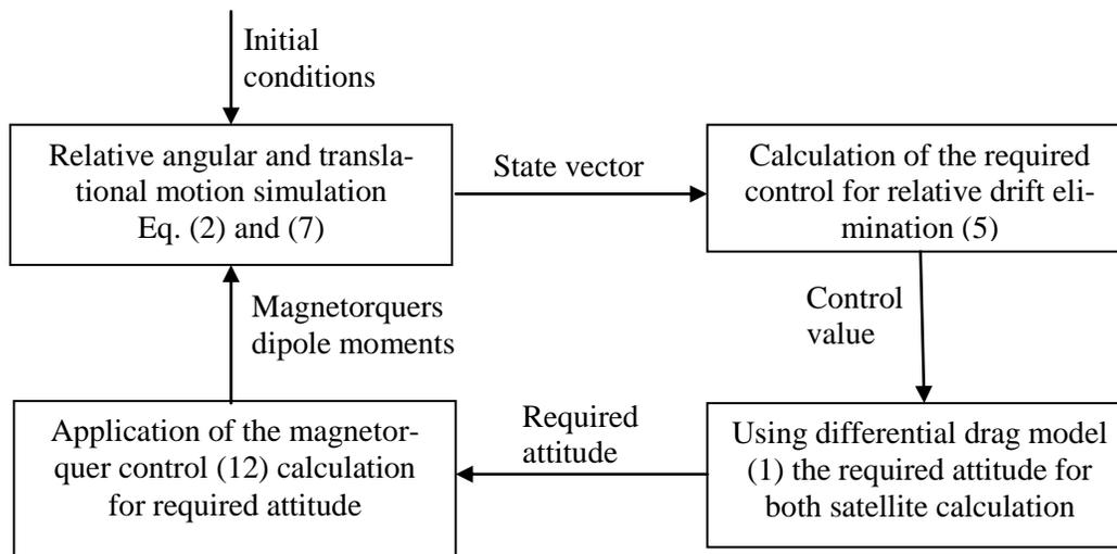
**Figure 3. Scheme of the control loop**
