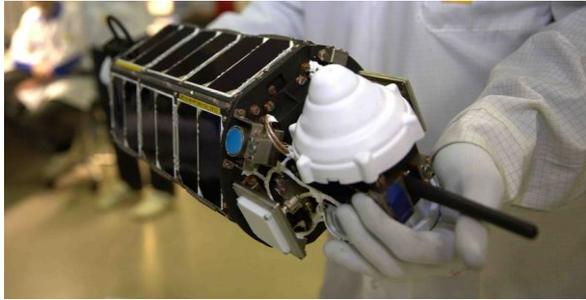
Fig. 3. TNS-0 nanosatellite platform
